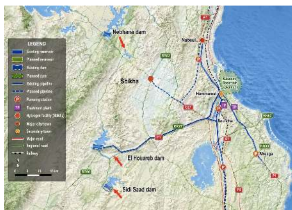
Figure 4. Water infrastructure potentially supplying the Sbikha hydrogen facility.
